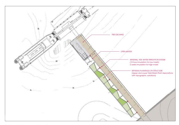
As the marsh planters were developed in response to the river conditions, instead of being submerged, where strong currents would damage the plantings, they were raised slightly above high tide.
